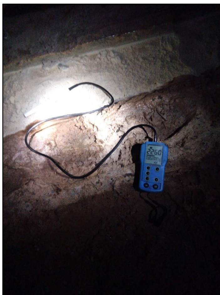
Figure 49: Multi-parameter probe collecting field parameters in a drain stream underground.
